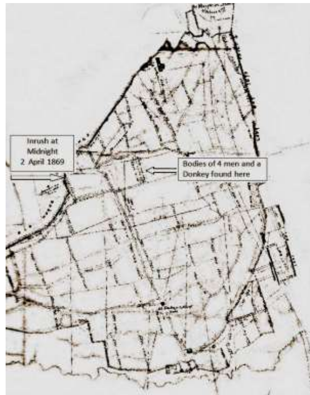
Plan of Molyneux Colliery showing location of worked areas, inrush and location of bodies.
